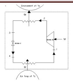
Fig: 1a. Schematic Diagram of an Industrial Ice Plant
