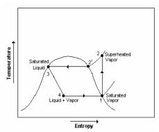
Fig: 2. T-s Diagram of Single Stage Vapour Compression Cycle
